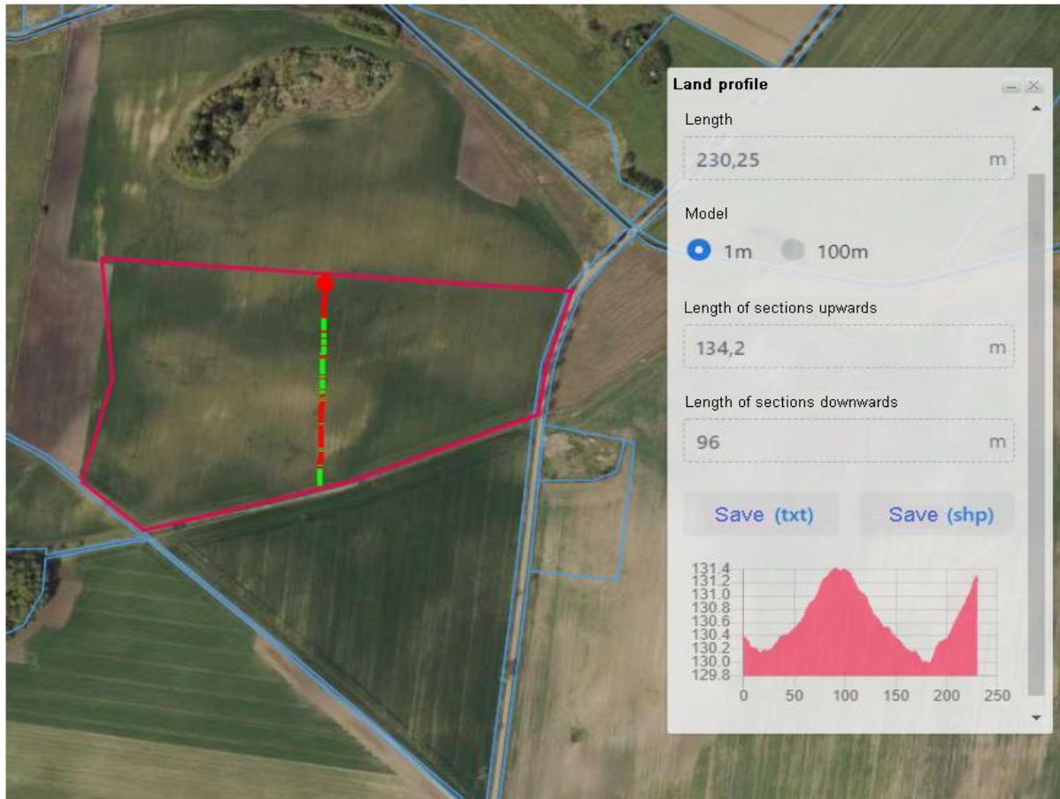
Fig. 4. Land profile of the project area for the photovoltaic farm
